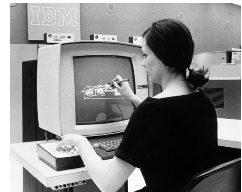
Design Augmented by Computer (DAC-1) running on an IBM 2250 graphics console, 1964
